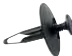
Trim Attachment Rivet - Screw Type Various Interior Black Plastic; 6.3 mm Hole; Flange: 25 mm; Panel Range 2-12 mm Ford Taurus/Sable 2000+
