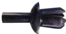
Air Intake Cowl Grille Rivet - Drive Type; Plastic Hole: 4 mm Panel Range: 6 mm; Flange 9 mm Mercedes, Volvo
