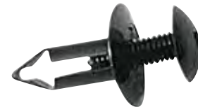
Rivet Cowl Panel to Reinforcement Plate Hole: 6 mm; Panel Range: 2 - 8 mm Washer Face: 14 mm Datsun Truck '80+ Infiniti '91+
