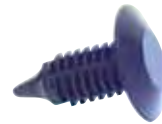
Retainer, Trim Panels; Black Plastic Hole: 7.9 mm; Head: 19 mm; Stem Length: 23 mm; GM Saturn '91+, Chrysler Mini Vans '87+ GM C/K Trucks '99+
