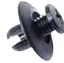
Cowl Vent Rivet - Screw Type; Black Plastic Fender Splash Shield and Air Ducts Hole: 8 mm; Grip Range: 2 - 5 mm; Washer Face: 20 mm; Honda, Mazda, Nissan '84+
