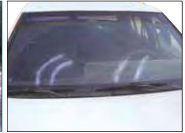
Mechanical Glass Damage
