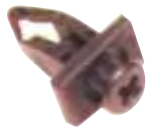
Rivet - Screw Type Cowl Grille Black Plastic 6 mm Sq. Hole; 8 mm x 12 mm Head Grip Range 5 mm - 7 mm Nissan 300ZX '90+
