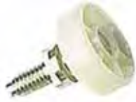
Quarter Window Regulator Roller; 15/16" Dia.; 5/16" Thick Ford '71+
