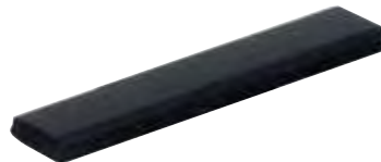
3/8" x 1/2" x 1" 80 Durometer Neoprene Rubber Windshield Setting Blocks For Use on Vehicles Without Support Brackets
