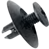
Rivet - Screw Type; Plastic Hole: 6 mm; Panel Range: 2 - 5 mm Washer Face: 20 mm Nissan, Isuzu, Mazda, Various Applications
