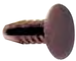
Retainer - Cowl Grille Black Plastic; Hole: 5 mm Head Dia.: 12 mm; 15 mm O/L Nissan 240SX '90+
