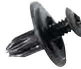
Rivet - Screw Type, Air Scoop Grill (Cowl Vent Panel); Black Plastic Hole: 6 mm; 2 - 6 mm Panel Range; 18 mm Washer Face Honda Prelude '83+
